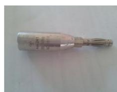
Fig.1.6 Sealed Alpha Source Holder
