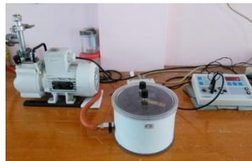
Figure (4.6) Experimental Setup of Alpha Radiation Detection
